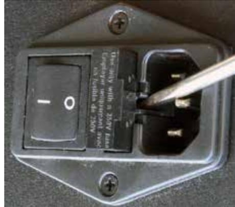
3. The fuse holder contains 2 fuses. The top one is a spare and can replace the blown one at the bottom.
