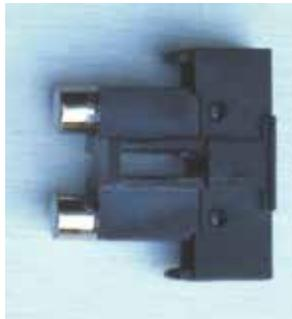
4. Replace fuse holder into power connector by making sure that good fuse is at bottom. Replacement fuses should be rated:
